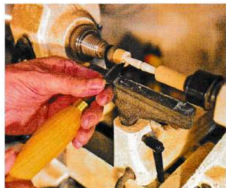
30 A small toggle is turned on the lathe
