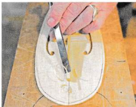
12 The front braces are scalloped and gabled
