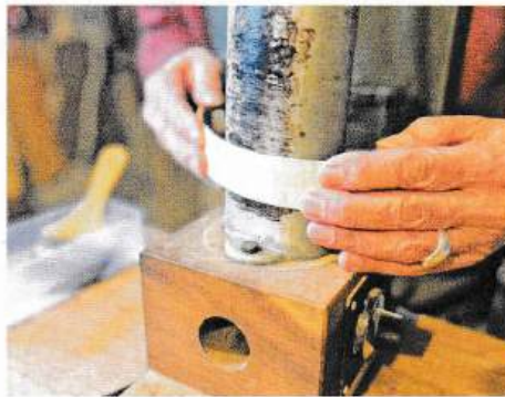
8 Bending the sides on a heated iron
