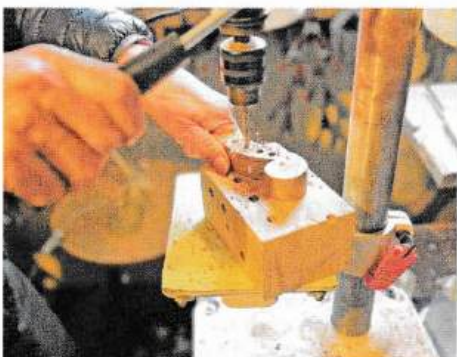
14 Drilling the peg holes
