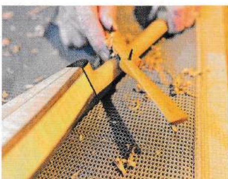
24 A spokeshave is useful for slimming down the neck
