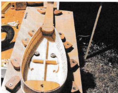
17 Soundboard, ribs and neck in place on the work board
