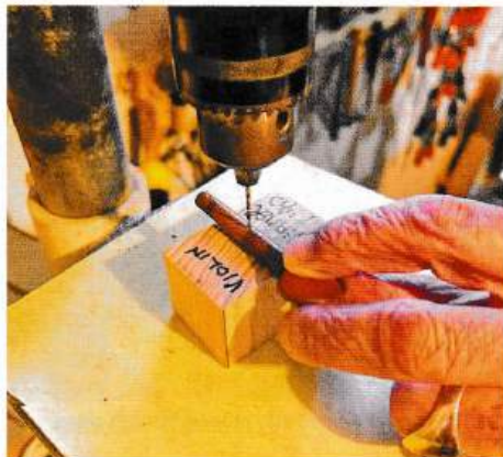
26 String holes are drilled into the pegs
