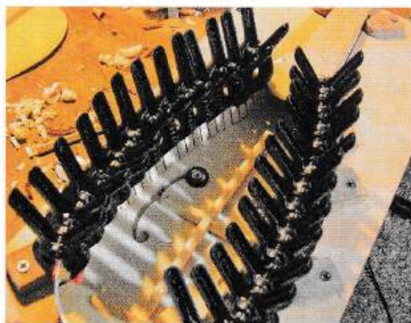
18 The back linings held in place with clamps
