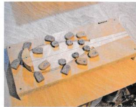
9 Tail block in place on the work board
