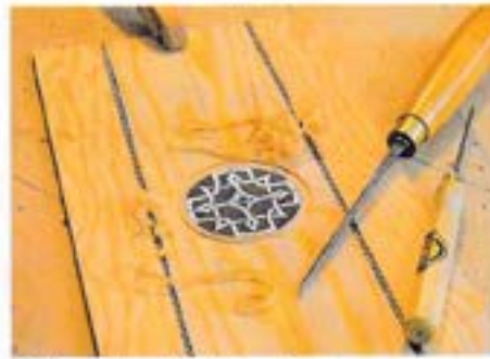
10 The rosette channel is cut
