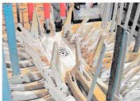
19 Cramping the soundboard in place
