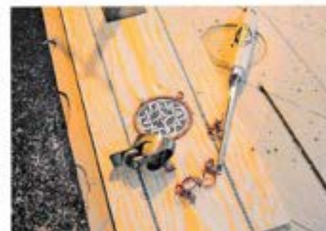
12 Using a thumb plane, the rosette is levelled
