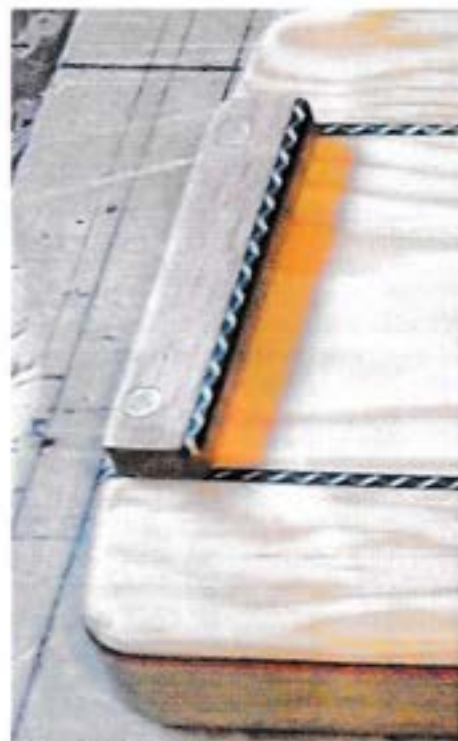
25 The tie block in place
