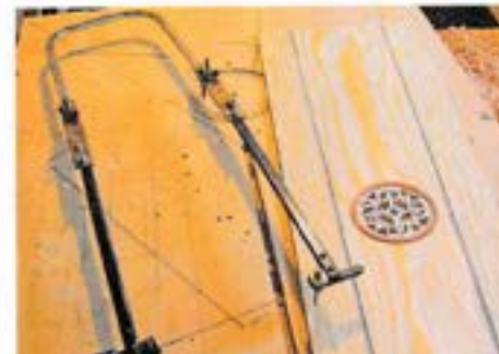
13 The sound hole pattern is cut out with a 'long reach' fretsaw...
