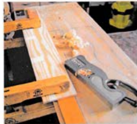
6 Soundboard edges being squared
