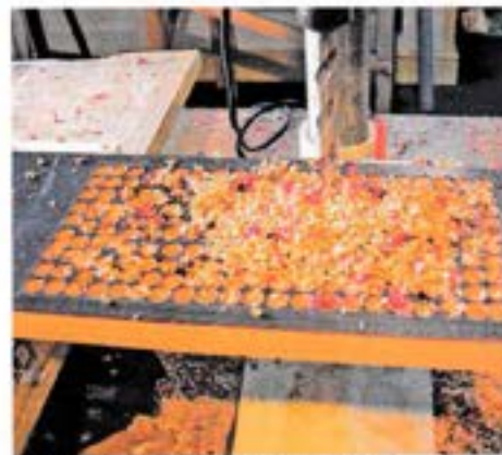
3 Drilling out waste from the sound box
