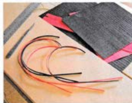
11 2mm wide veneer strips are used to make up the rosette
