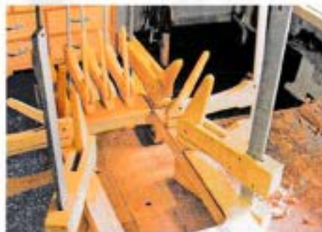
20 Mahogany trims for the remaining front are placed in cramps
