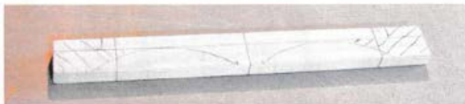
18 Marking out the soundboard support
