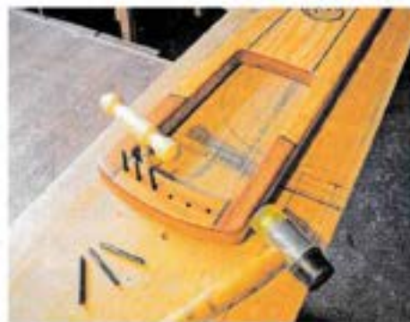
26 Screwing in the wrest pins
