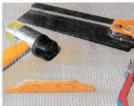
27 The small bridge is made from mahogany
