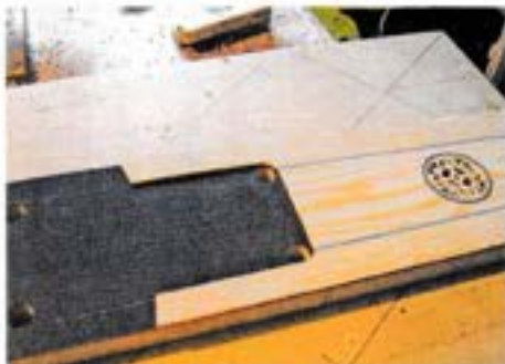
15 Achieving the correct soundboard shape
