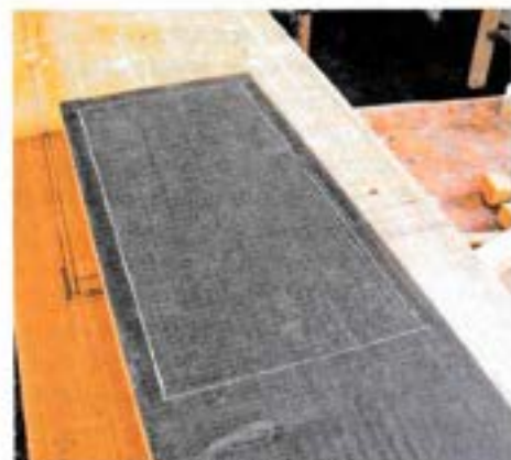
2 Veneers attached to the lyre's body
