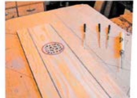
14 ... and finally cleaned up with needle files and a small chisel
