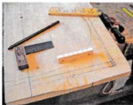
24 The tie block holes once marked out
