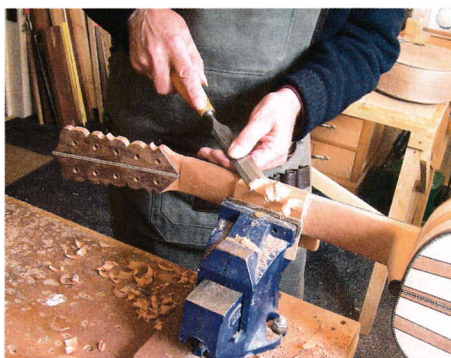
92 Final shaping of the neck with a chisel...
