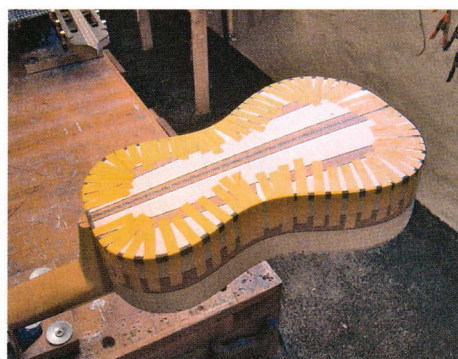
77 Masking tape holds the bindings in as the adhesive cures
