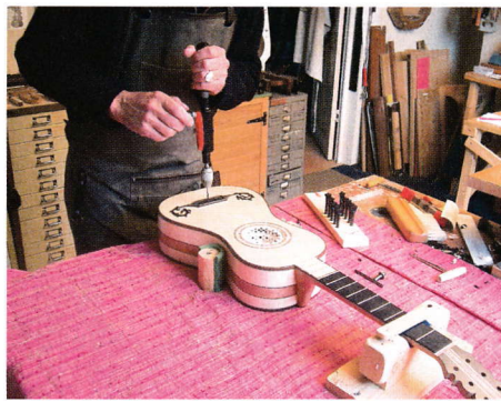
89 Drilling down through the bridge is a life shortening moment...
