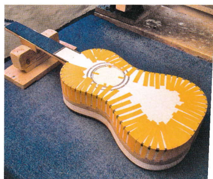
78 Masking tape also holds the front bindings in
