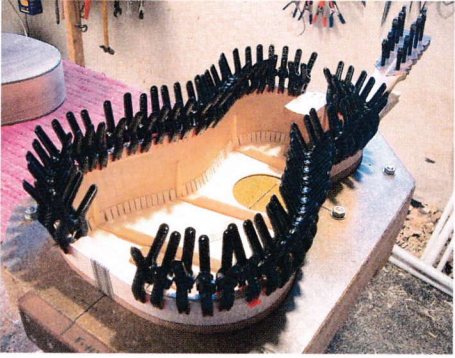
67 The kerfed lining is held in place with mini clamps
