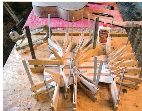
62 The four back braces are cramped into place
