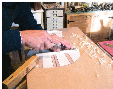
64 The ends of the back braces are scalloped
