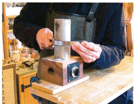
76 Bending the bindings on the hot iron
