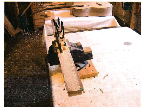
63 The back braces are curved on a sanding stick
