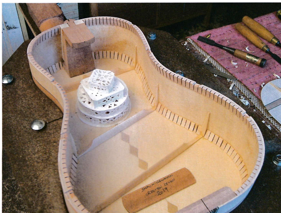
61 The completed rose is fitted
