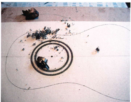
42 A thumb plane helps to level the hoops
