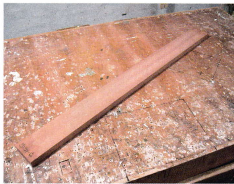
5 The 1m long mahogany billet used to make the neck
