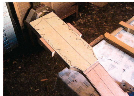
16 Avoiding splits on the edges of the headstock
