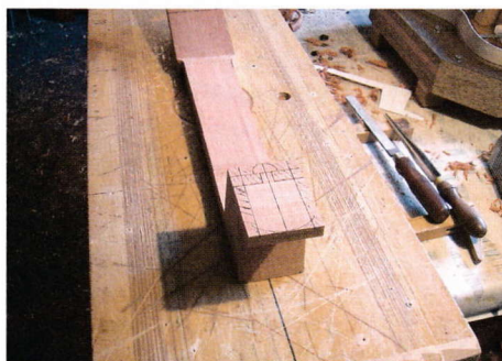
8 The slipper heel marked out
