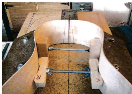
34 The tapered rib ends are marked out
