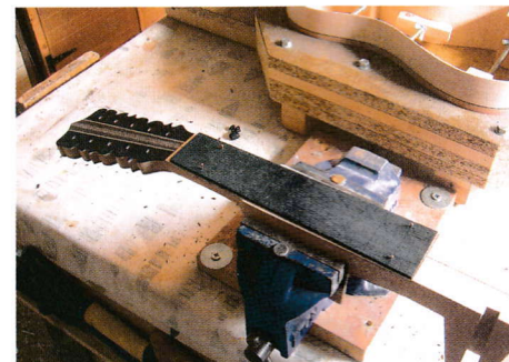
26 The fingerboard pinned in place
