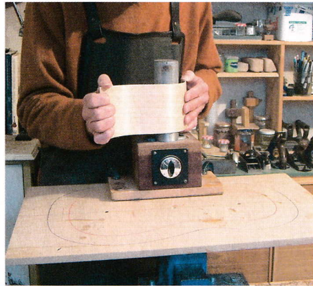
30 Bending the ribs on the hot iron
