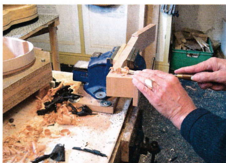
10 The heel slot is chiselled out
