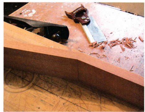
6 A scarf joint cut at 14° for the headstock
