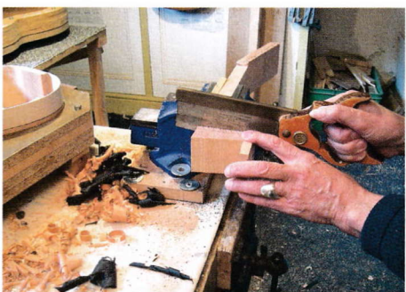
9 A dovetail saw is used to cut out the slipper heel
