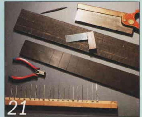
The fingerboard in stages, with the frets roughly cut to size
