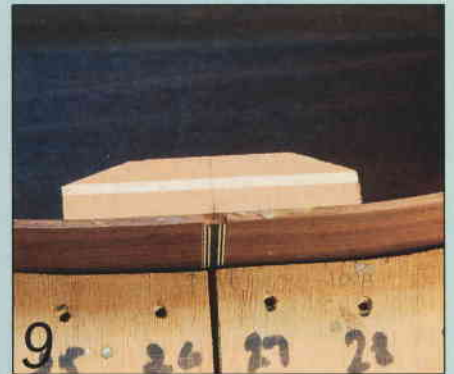
9 The tailblock fitted; an inlay can be added if desired
