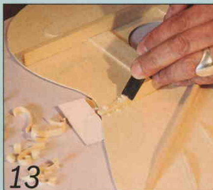
13 The ends of each strut and harmonic bar must be scalloped into a curve
