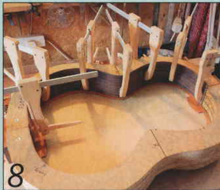
8 Once bent, the curved side sections are clamped into the mould
