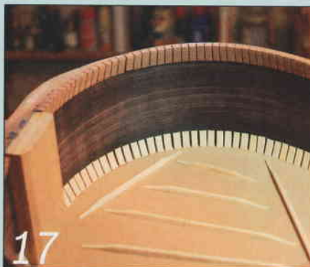
Small spruce triangles called tentellones hold the front in place
