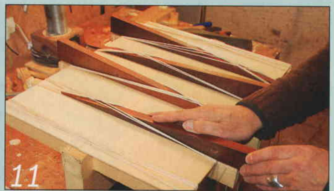
11 The two halves of the front are butt-jointed in the lace-and-wedge jig
