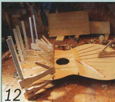
12 The front bracing struts are held in place with cam cramps
