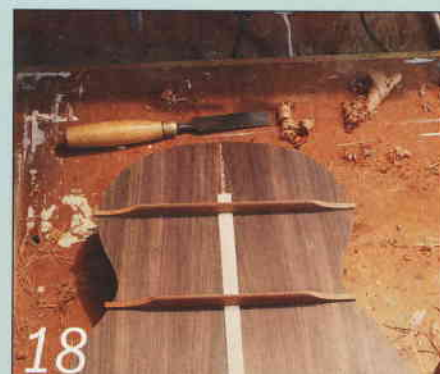
The mahogany back braces are fitted and their ends scalloped
