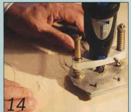
14 Cutting the rosette channel in the front is best done with a mini-router
