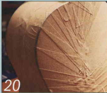
Bindings and purflings are held in place with masking tape
