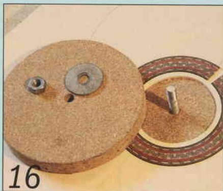
The simple chipboard jig that cramps the rosette in its channel
