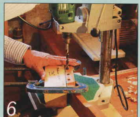
6 The machine head housings must be bored accurately
