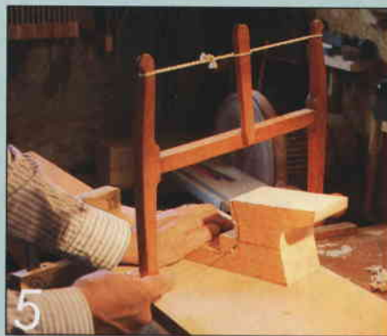
5 The shape of the heel is roughly cut with a bowsaw
