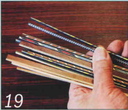
Examples of ready-made bindings and purflings - another component that's worth buying
