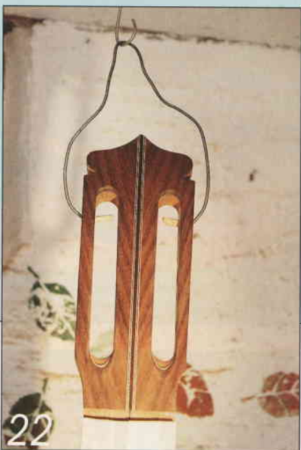
A wire hanger is a handy accessory to help the finishing process
