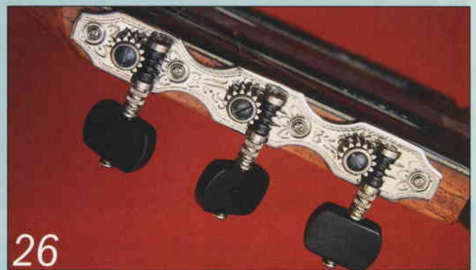
The machine heads are fitted into their housings in the headstock
