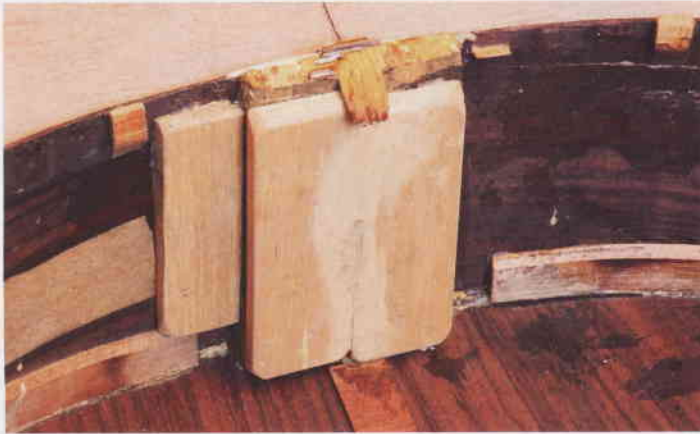
▲ Pic14 The tail block had been crudely strengthened with old pieces of spruce which offered next to no support
