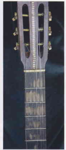
▲ Pic.3 The fingerboard had been badly worn down and the machine heads had all but seized up
