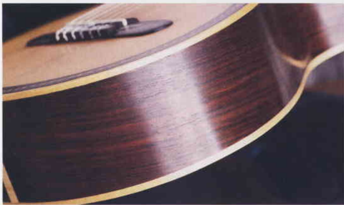
▲ Pic.22 Fresh bindings, made from an old maple floorboard, in place
