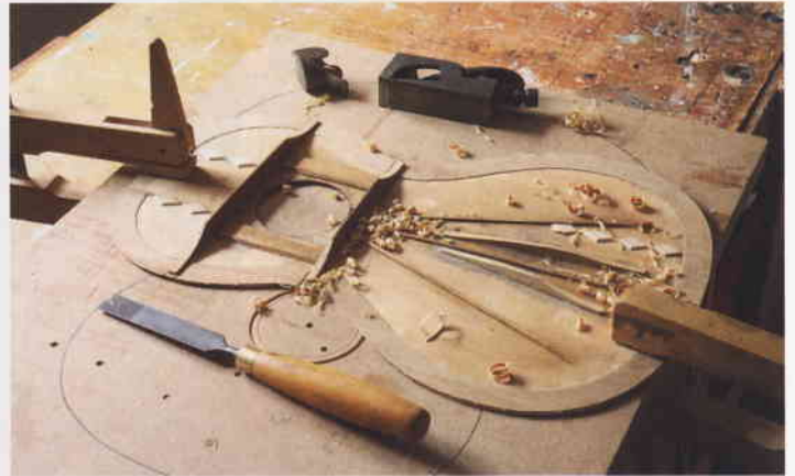
▲ Pic15 The edges of the top were strengthened with 1mm ply and cracks were cleated with spruce. Old braces were trimmed to improve sound
