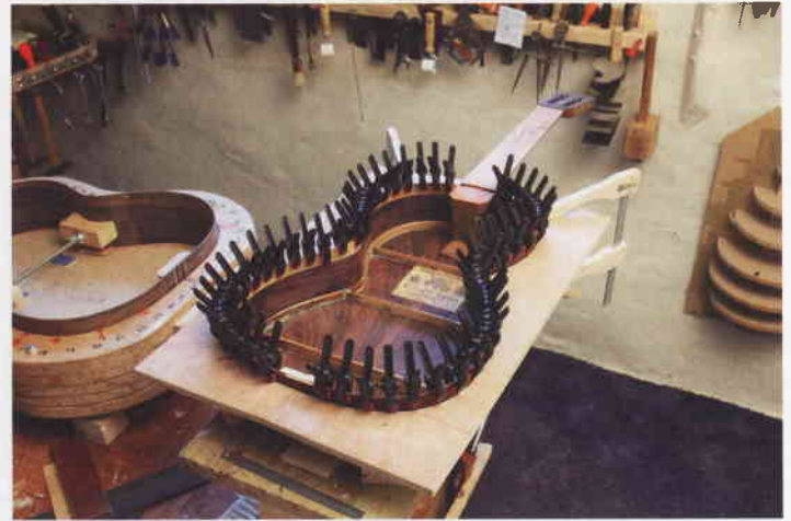
▲ Pic17 The ribs were strengthened with 1mm ply strips held in place with mini clamps
