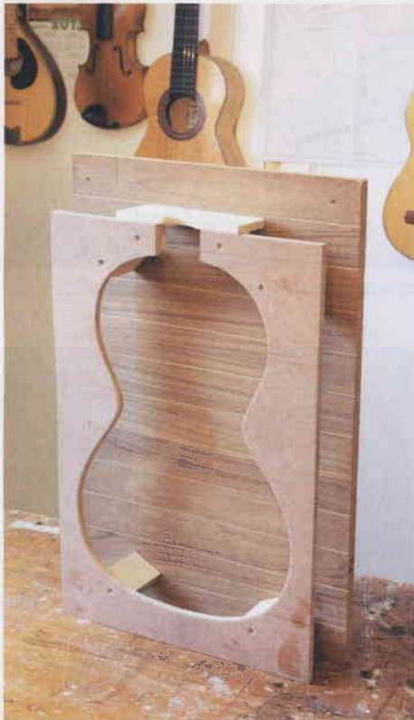
▲ Pic.4 The cradle, made from plywood and pine blocks, kept the structure of the instrument intact during surgery
