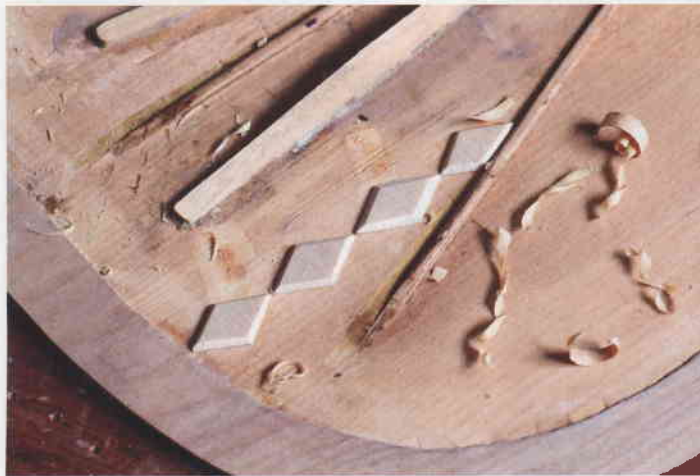
▲ Pic16 A detailed view of spruce cleats cross banded for strength
