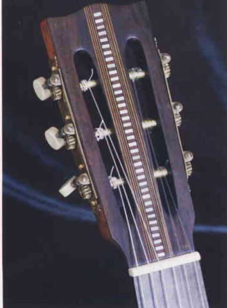
▲ Pic.25 The headstock polished and the machine heads freed and buffed
