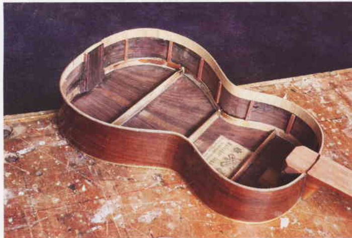
▲ Pic18 The inside was now clean, with a rosewood tailblock support, rosewood braces and 1mm ply edge strengtheners
