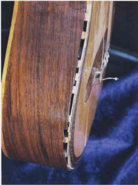
▲ Pic.1 Splits in the side and cracks in the front were an early sign of what lay ahead
