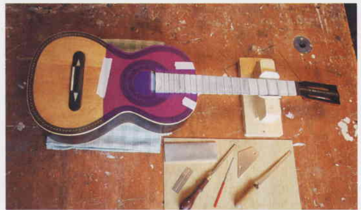
▲ Pic.23 The frets were fitted, trimmed, levelled and polished
