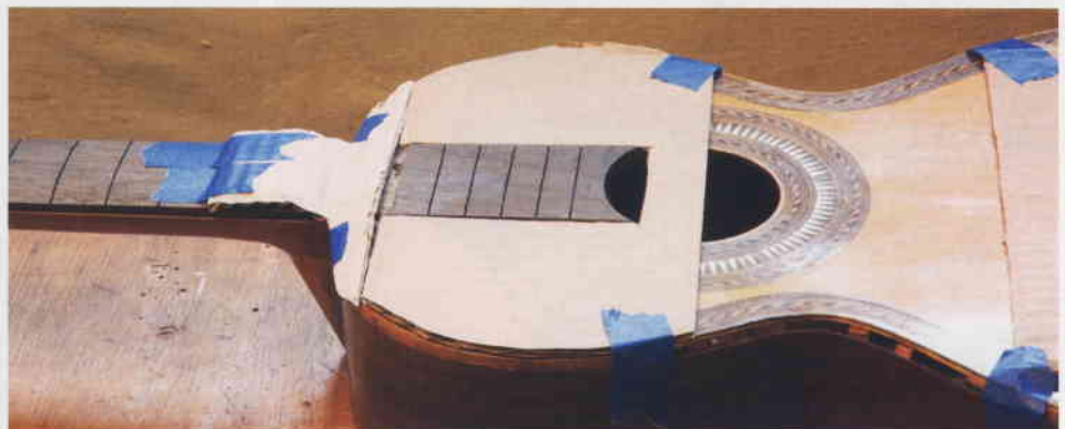
▲ Pic.6 Protective cardboard guards prevented scorching of the rosette and purflings during fingerboard removal
