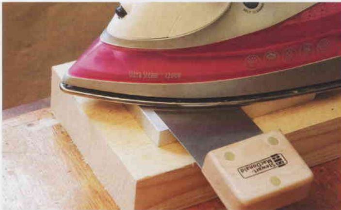
▲ Pic7 A domestic iron was used to heat both an aluminium slab and a spatula to aid removal of the fingerboard and bridge
