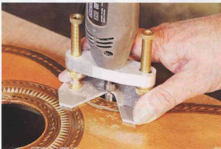
▲ Pic11 A Dremel mini-router was used to cut out the old bindings before removing the top
