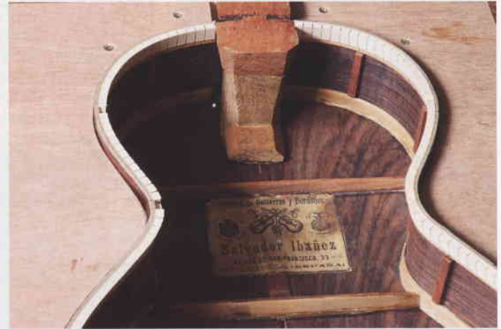
▲ Pic19 A kerfed lining was put into place and levelled to receive the top
