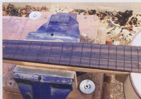
STEP 5. The fingerboard pinned dry onto the neck
