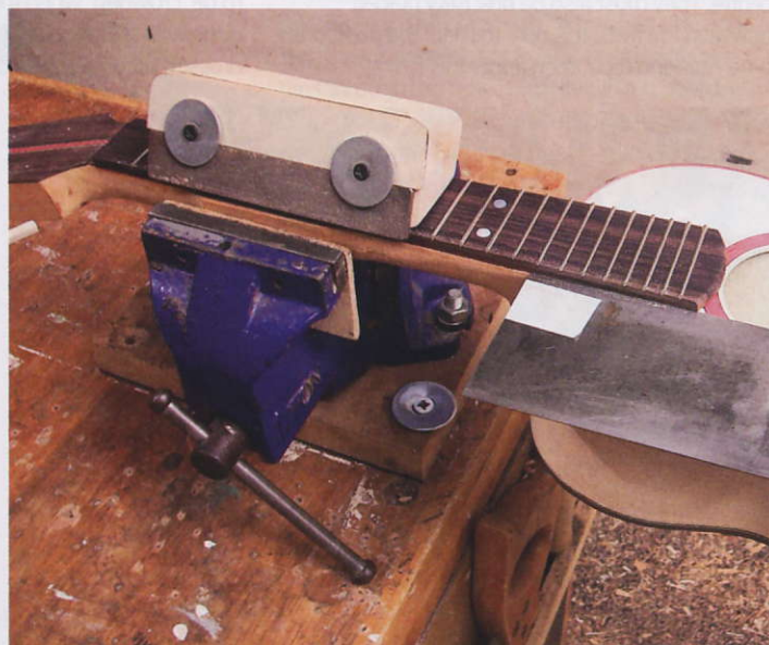
STEP 11. Bevelling the fret ends
