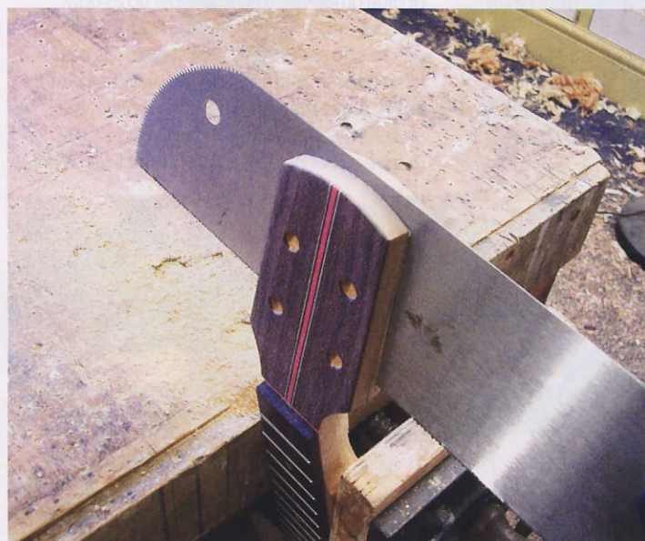
STEP 13. Cutting the headstock to the correct thickness
