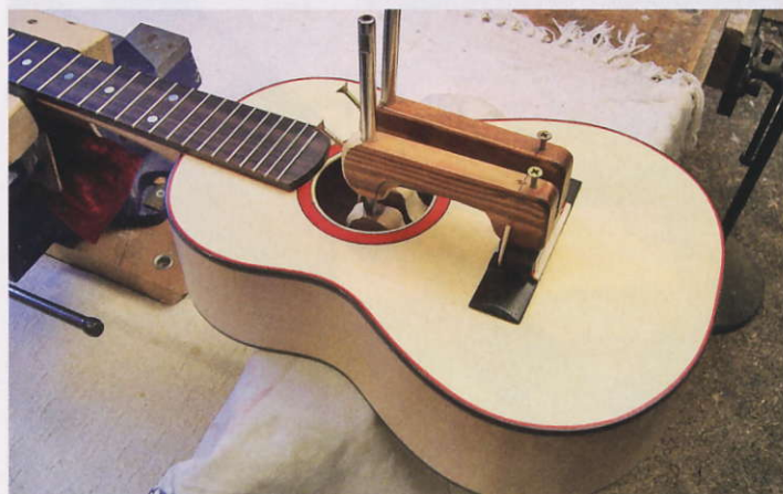
STEP 19. Clamping the bridge into place
