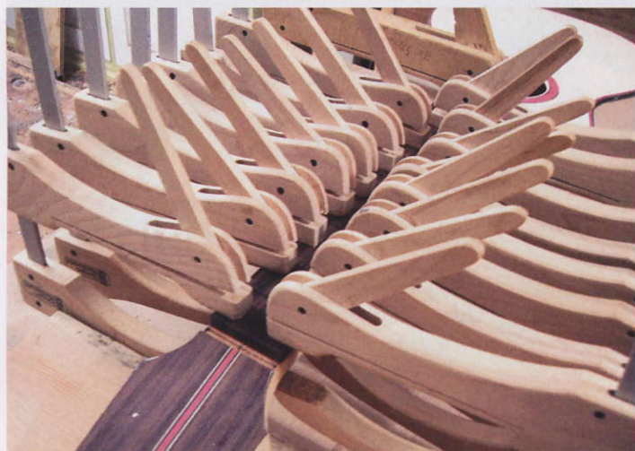
STEP 6. Clamping the fingerboard into place
