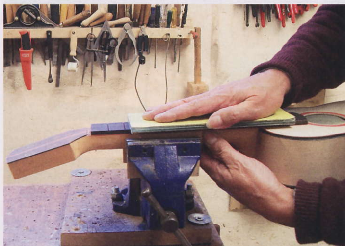
STEP 7. Levelling the fingerboard
