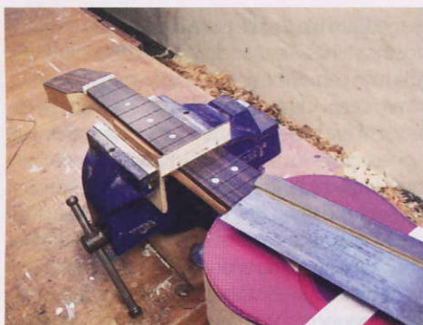
STEP 2. Checking fret slot depths
