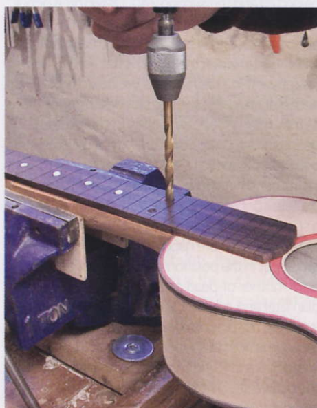
STEP 9. Drilling the position dot housings
