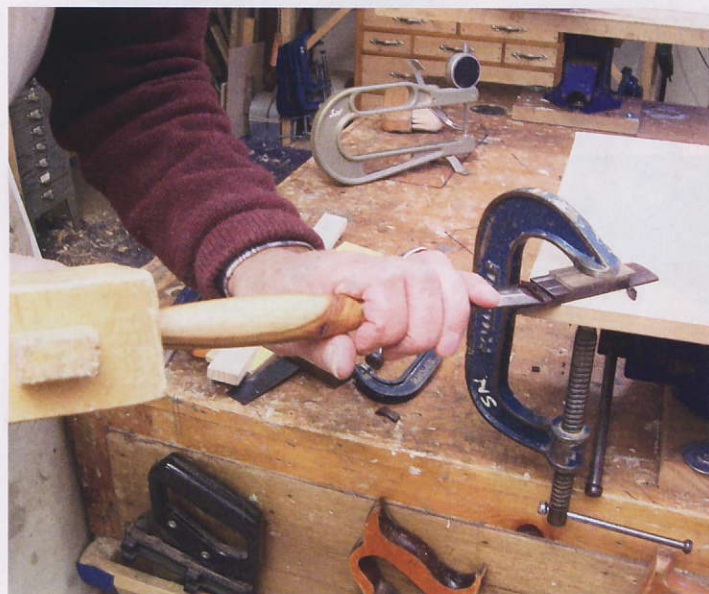
STEP 15. Reducing the thickness of the bridge wings
