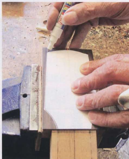
▲ Pic.25 Marking the final headstock shape out
