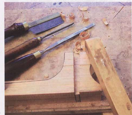
▲ Pic.19 The wedge slots chiselled out
