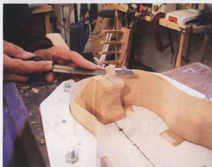
▲ Pic.30 Wedges are cut flush
