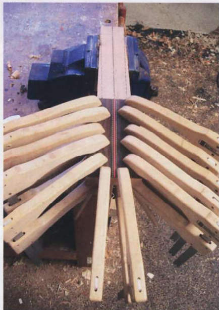
▲ Pic.24 The headstock cover glued on
