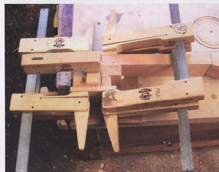
▲ Pic.16 The heel stack in clamps
