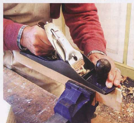
▶ Pic.9 Planing the bottom edge of the sides
