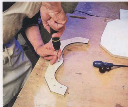
▲ Pic.5 Attaching the template onto a side piece
