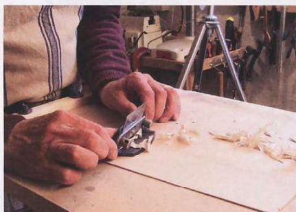
▲ Pic.10 The No.080 cabinet scraper in use
