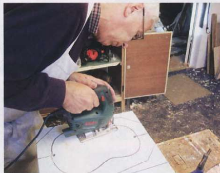
▲ Pic.2 Components of the mould marked onto chipboard
