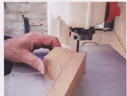
▲ Pic.17 Cutting the 'slipper' on the bandsaw
