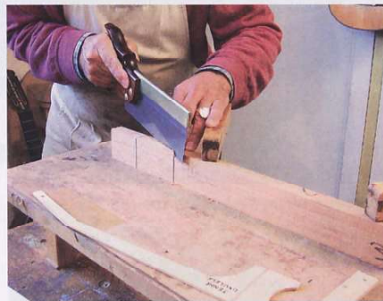
▲ Pic.14 Cutting the headstock scarf joint
