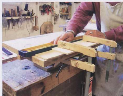
▲ Pic.31 The soundboard edges made true
