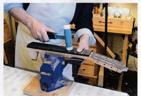
95 Tapping frets in with a soft-faced hammer
