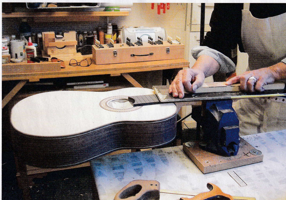
94 Levelling the fingerboard with a plate glass sander
