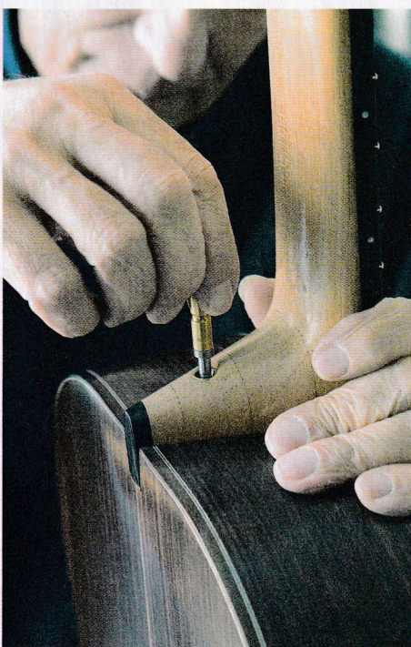
105 Assembling the guitar with a Halsschraube
