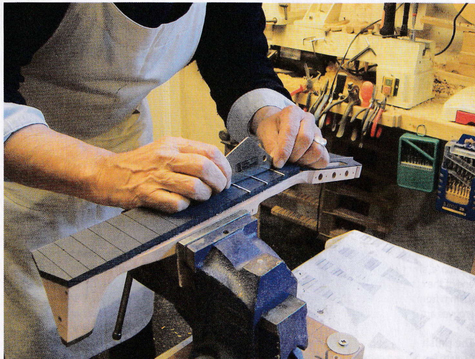
97 Checking the frets are level
