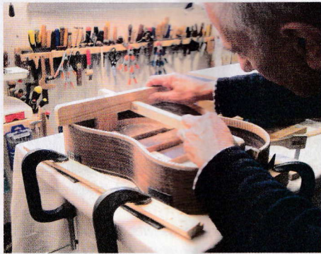
70 Testing the tops of the ribs for flatness
