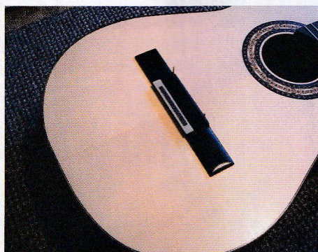
84 Cocktail sticks help to prevent the bridge from sliding out of line
