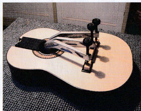
85 Bridge clamped into place
