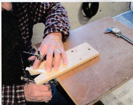
80 Cutting a hole in tie block bone with a pearl saw
