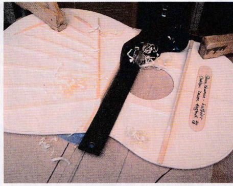
68 Gabling the harmonic bars
