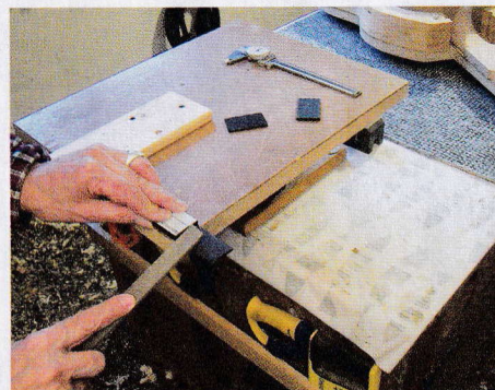
78 Rounding bridge wings with a sanding stick
