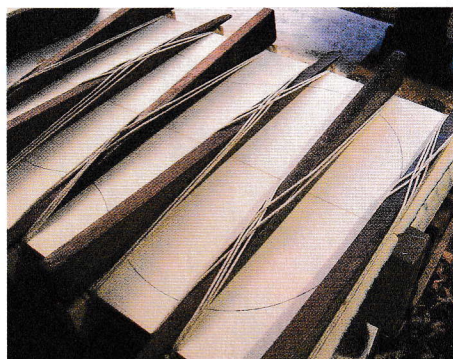
58 The soundboard in the wedge and lace jig
