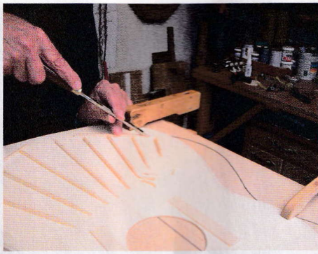
67 scalloping the fan brace ends
