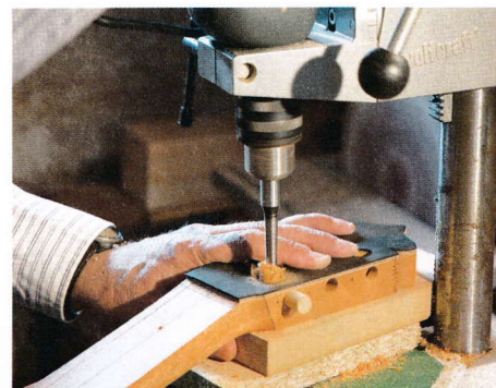
47 String slot holes being drilled
