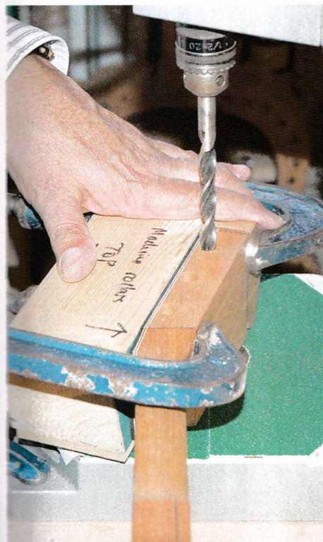
46 Drilling tuner roller holes
