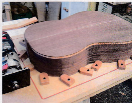
34 Binding/purfling channels cut into the back
