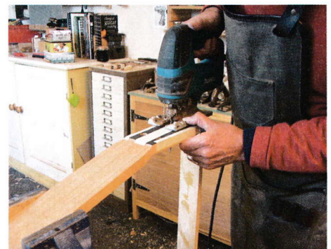
48 Jigsawing string slots
